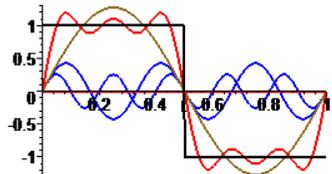
$$\text{Ordre 5 : } S_F(t) = \frac{4}{\pi} \left( \sin(\omega t) + \frac{1}{3} \sin(3\omega t) + \frac{1}{5} \sin(5\omega t) \right)$$
