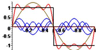
$$\text{Ordre 7 : } S_F(t) = \frac{4}{\pi} \left( \sin(\omega t) + \frac{1}{3} \sin(3\omega t) + \frac{1}{5} \sin(5\omega t) + \frac{1}{7} \sin(7\omega t) \right)$$
